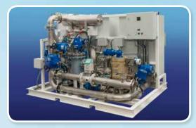
An innovative ballast water treatment system with capacities from 34m³/h to 1,200m³/h with IMO and AMS approval. Combines filtration and UV technology to kill micro-organisms and pathogens. The new Cathelco Evolution BWT system is being tested for U.S. Coast Guard Type Approval under the 'live/dead' standard.
