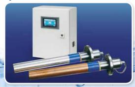
Eliminates blockages in seawater pipework caused by the growth of barnacles and mussels. Copper and aluminium anodes installed in seachests or strainers are wired to a control panel. Does not interfere with reverse osmosis systems.
