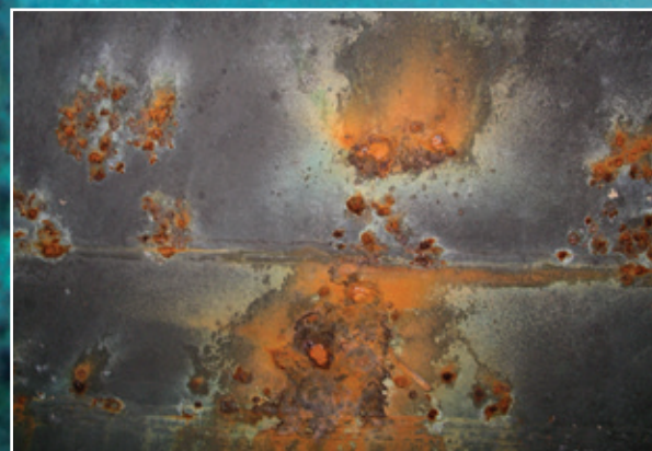
Corrosion 'blisters' on hull plate.
