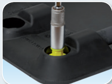
2 Nut is tightened using ordinary wrench. Top section breaks off when correct torque is achieved.
