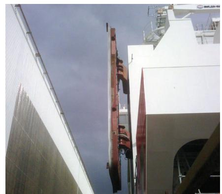
Hydraulic operated locking pins are used to secure the door to suit the weather tightness of the ROV door.
