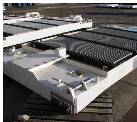
The hinges are fitted with bronze bearings. Locking pins are used to secure the moonpool top hatch door in the open and closed position. Indication lights are placed on the control box to monitor the safe operation of the top hatch door. As an option, signals can be send to a bridge indication panel or to the LARS operation system.
